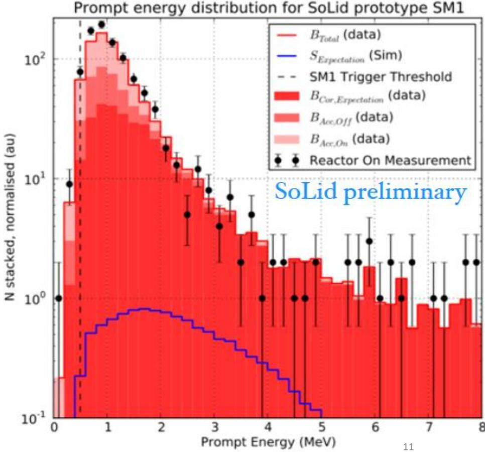
Background spectrum measurement used for re-evaluation of SoLid sensitivity
