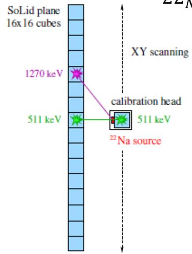
$^{22}\text{Na}$  Compton edge of 1270 keV gamma used for LY measurement
