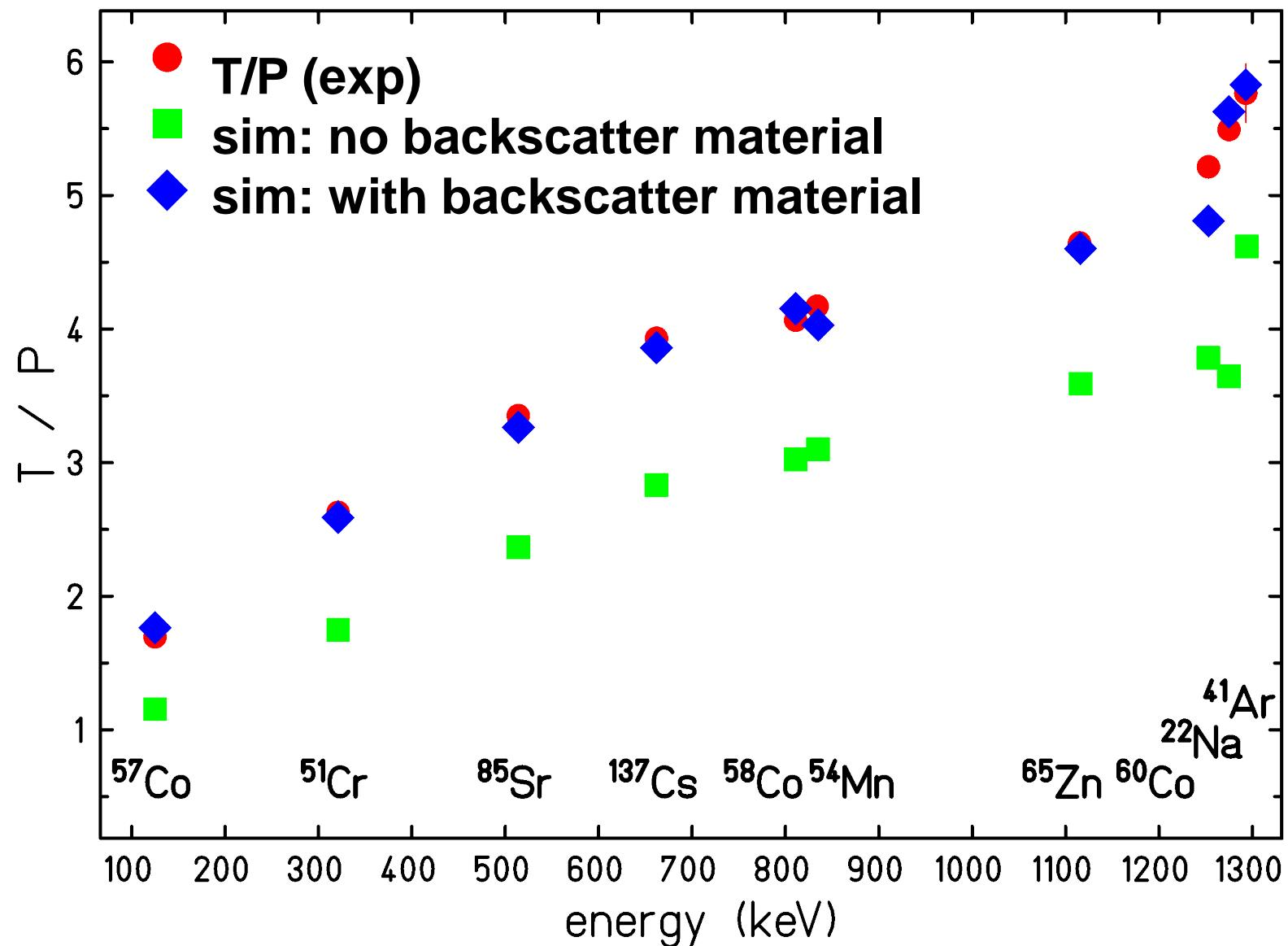
● ● ● Calibration of germanium detector: absolute efficiency
