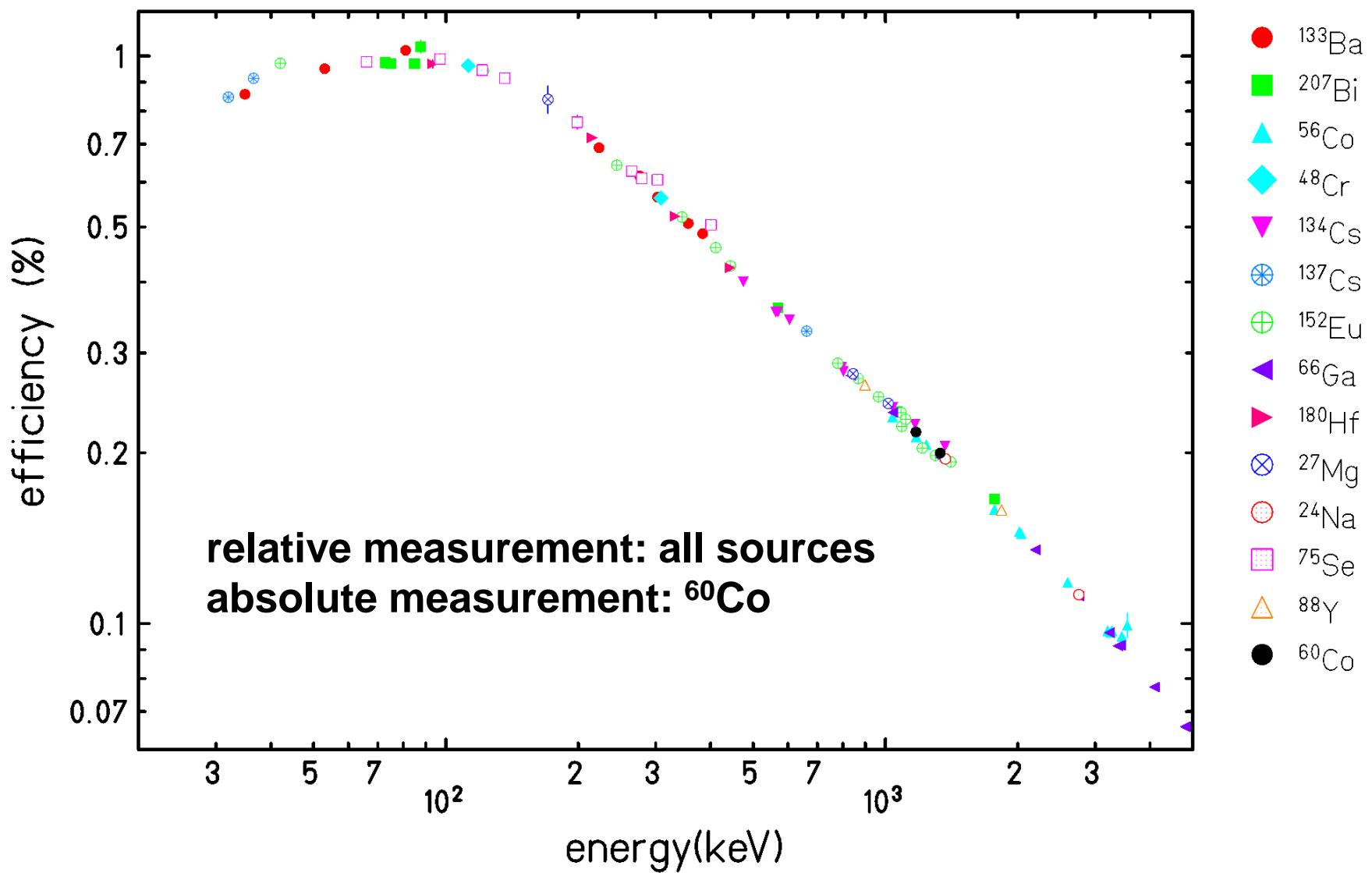
● ● ● Calibration of germanium detector: absolute efficiency
