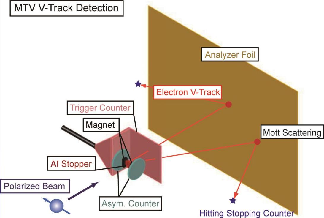
Transverse Polarized  ${}^8\text{Li}$   $\sim 10^7$  pps – 80% pol. @ 30keV
