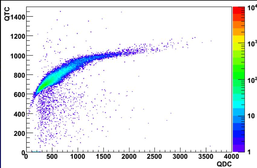
pQTC Charge readout using TDC
