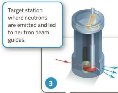
3 Target station where neutrons are emitted and led to neutron beam guides.
