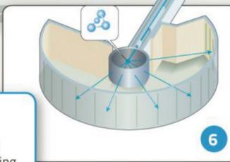
Instrument, where the neutrons scatter off the sample, hitting detectors and generating experimental data.
