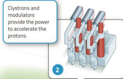
2 Clystrons and modulators provide the power to accelerate the protons.
