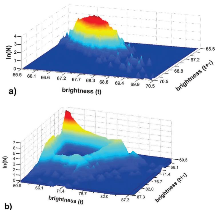
Fig 1 : Histograms reconstructed from time series of the FEM brightness (a) for a steady state just before a bifurcation point and (b) in the presence of oscillations. Highly probable states are represented in red, and low-probability states are in blue.
