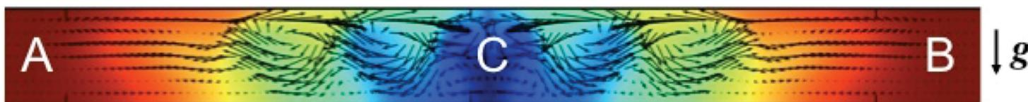
*Fluid velocity field superimposed on the density field (red: high density, blue : low density). Upon reaction between A and B, C is produced in the middle of the system, increasing the surface tension and inducing thereby a convergent Marangoni flow at the surface and hence a vertical down-flow. By decreasing the local density of the solution, C generates an antagonistic vertical up-flow opposing the Marangoni-induced flow. This competition induces sustained oscillations.*
