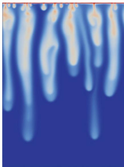
Figure: Numerical convective dissolution of CO<sub>2</sub>-rich fingers in a reactive host phase.
