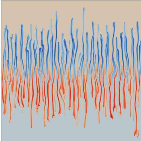
Figure: Numerical convective fingering pattern obtained when a denser solution lies above a less dense solution in the gravity field and differential diffusion effects are at play.
