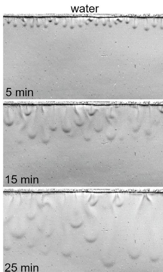
Figure: Convective dissolution pattern of CO<sub>2</sub> dissolving in an aqueous salt solution, visualized with the help of a Schlieren imaging system sensitive to density gradients in the solution.
