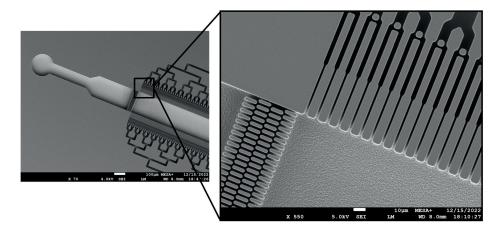
Figure 4. Silicon etched device produced by medium-range UV photolithography and cyclic deep reactive ion etching for the experimental exploration of the possibilities of the novel Hydrodynamic Chromatography-Brownian Sieving (HDC-BS) nanoparticle separation scheme developed by our group.
