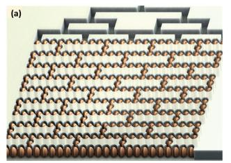
Figure 1. (a) Conceptual image showing the principle underlying the new concept wherein a microgroove template is used to perfectly organize arrays of chromatographic particles.
