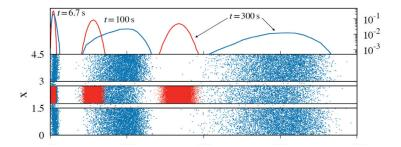
Figure 3. Lagrangian particle flow simulations of the separation of a mixture of 100 and 200 nm particles using the Hydrodynamic Chromatography-Brownian Sieving (HDC-BS) principle developed by our group.
