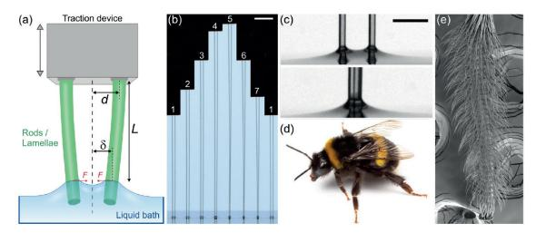
(a) Schematic of the experimental setup where two partially immersed slender structures with a dry length L are clamped at a distance 2d to a traction device and deflected by the capillary force F induced by the menisci. (b) Snapshots of an experiment cycle where two rods coalesce when the dry length is large enough
