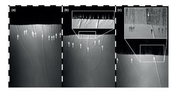
Schlieren images of the convective dynamics for an ice thickness of (a) 30 mm, (b) 50 mm, and (c) 80 mm when a 35 ppt NaCl solution is cooled at -20° C from above in a chamber kept at 0° C. The dark region at the top is the ice layer, and the gray area is the underlying water. Long streamer positions are marked with solid arrows while the zoom insets in (b) and (c) also indicate short finger positions with dashed arrows.
