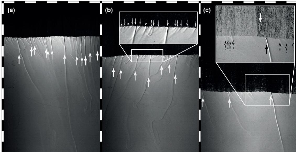
Schlieren images of the convective dynamics for an ice thickness of (a) 30 mm, (b) 50 mm, and (c) 80 mm when a 35 ppt NaCl solution is cooled at  $-20^{\circ}\text{C}$  from above in a chamber kept at  $0^{\circ}\text{C}$ . The dark region at the top is the ice layer, and the gray area is the underlying water. Long streamer positions are marked with solid arrows while the zoom insets in (b) and (c) also indicate short finger positions with dashed arrows.
